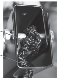
Double knot around bolt
