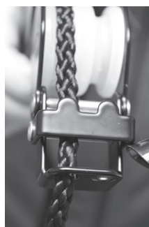
Proper rope placement in brake
