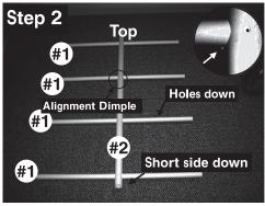
4 Horizontal Crossbars (#1) inserted through 1 Center Vertical (#2) Note: Slide horizontal crossbar into left side of center vertical following direction of arrow until alignment dimple meets center vertical. (see enlargement)
