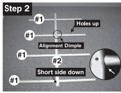
4 Horizontal Crossbars (#1) inserted through 2 Center Vertical (#2) Note: Slide horizontal crossbar into right side of center vertical following direction of arrow until alignment dimple meets center vertical. (see enlargement)
