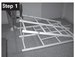
Insert Bottom Sliderails (**#8**) into Front Grid Assembly and fasten *(making sure fully inserted)* using **2**- #08 x 3/4" Fastening Screws (**#1**) **Note: Fasteners in Bottom Hole Only**
