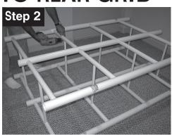
Insert and fasten next 3 rows of Sliderail to Front Grid using 6 - #08 x 3/4" Fastening Screws (#1) **Note: Fasteners in Bottom Hole Only**
