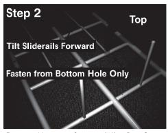
Fastening Horizontal Sliderails (**#8**) in Rear Grid using **8** - #08 × 3/4" Fastening Screws (**#1**) **Note: Start at top row and work down.**
