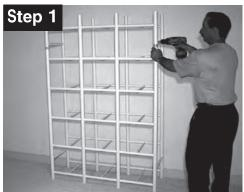
Fasten 4 Front & Rear Grid Connecting Tubes (#5) to Front Grid Assembly Using 4 - #06 x 1/2" Fastening Screws (#1)
