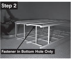
Insert and fasten 18 Horizontal Sliderails (#7) into Front Grid Assembly using 18 - #06 x 1/2" Fastening Screws (#1) Note: Fasteners in Bottom Hole Only, Work from Bottom Row to Top Row Making Sure All Tubes are Fully Inserted!
