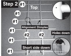
6 Horizontal Crossbars (#1) inserted through 2 Center Verticals (#2) (holes facing down) Tip: When installing second Center Vertical, stand assembly with Horizontal Crossbars placed on floor and push down second Center Vertical to Alignment Dimples.
