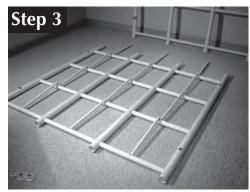
All Horizontal Sliderails fastened to Rear Grid Note: Fastener in Bottom Hole Only
