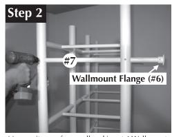
Move unit away from wall and insert 4 Wallmount Extension Tubes (#7) at 4 Locations. Fasten With 8 - #08 x 1-1/2" Extension Tube Fastening Screws (#2)
