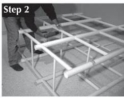
Insert and fasten next 3 rows of Sliderail to Front Grid using 9 - #08 x 3/4" Fastening Screws (#1) Note: Fasteners in Bottom Hole Only
