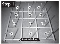
Horizontal Sliderails (#8) inserted in Rear Grid
