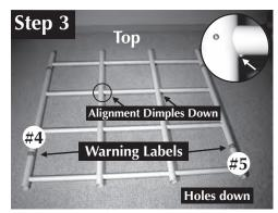
1 Left Front Corner Vertical (#4) and 1 Right Front Corner Vertical (#5)
