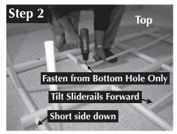
Fastening Horizontal Sliderails (#8) in Rear Grid using 12 - #08 x 3/4" Fastening Screws (#1) Note: Start at top row and work down
