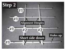
2 Center Verticals (#2) on 4 Horizontal Crossbars (#1) Tip: When installing second Center Vertical, stand assembly with Horizontal Crossbars placed on floor and push down second Center Vertical to Alignment Dimples.
