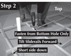
Fastening Horizontal Sliderails (**#8**) in Rear Grid using 12 -  $\#06 \times 1/2^{\parallel}$  Fastening Screws (**#1**) Note: Start at top row and work down Use only one fastener - Bottom Hole Only
