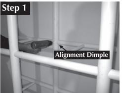
Fasten all Verticals to Horizontals. Make sure all joints are pressed firmly together, tight and against alignment dimples. 32 - #06 x 1/2" Fastening Screws (#1)
