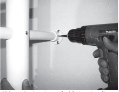
Slide unit back against wall while inserting all 4 Wallmount Extension Tubes (#7) into Wallmount Flanges (#6) and fasten with 4 - #06 x 1/2" Fastening Screws (#1).
