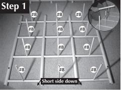
12 Horizontal Sliderails (#8) inserted in Rear Grid
