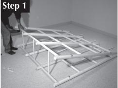
Insert Bottom Sliderails (**#8**) into Front Grid Assemble and fasten (*making sure fully inserted*) using 3- #06 x 1/2" Fastening Screws (**#1**) **Note: Fasteners in Bottom Hole Only**
